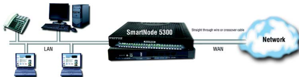
Figure 12. Connecting the SmartNode to the network
