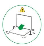
Put the rubber gasket on the back of endpoint, install the wall bracket (b) and lock the screws and gaskets
