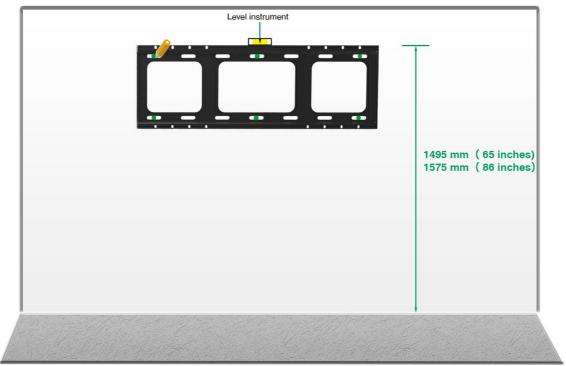
At least 6 screws for ETV65. At least 8 screws for ETV86.
