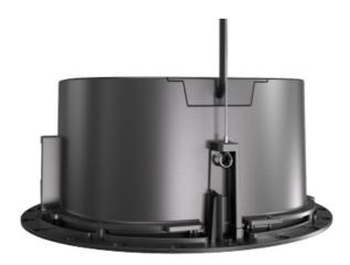
8. Thread the safety rope through the hole in the mesh cover; Wrap the safety rope around the support arm of the CS10; Then thread the safety rope through the washer; Use tweezers to secure the washer.
