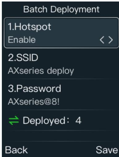
5. After successfully obtaining the Wi-Fi configuration, if there is a corresponding Wi-Fi in the environment, the deployment hotspot will be automatically disconnected and the available Wi-Fi network will be successfully connected.
