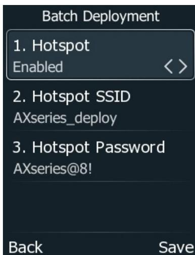
3. Press **Save**. At this point, the Handset A starts providing a hotspot for external connections.
