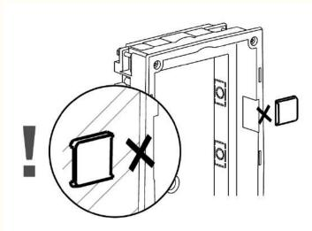
• Break off the side protrusions when the walling material has hardened.
