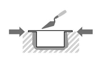
Make sure that the flush mounting box is slightly above the wall surface not aligning with the wall. A wrong installation may lead to water penetration and subsequent damage of the device. Use the side protrusions to achieve the proper flush mounting.
