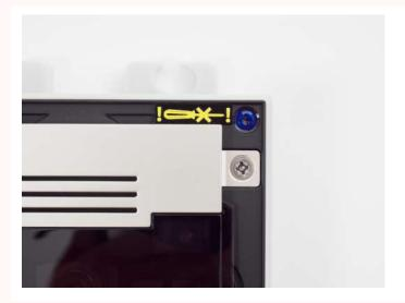
The main unit may not be removed from its base, so do not remove the marked resin-cast screw in the right-hand upper corner. Any screw tampering results in a loss of warranty.
