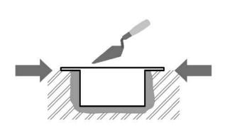
Make sure that the flush mounting box is slightly above the wall surface not aligning with the wall. A wrong installation may lead to water penetration and subsequent damage of the device. Use the side protrusions to achieve the proper flush mounting.
