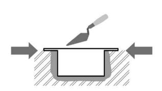
Make sure that the flush mounting box is slightly above the wall surface not aligning with the wall. A wrong installation may lead to water penetration and subsequent damage of the device. Use the side protrusions to achieve the proper flush mounting.
