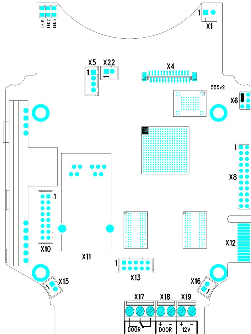
**Figure: 2N<sup>®</sup> Helios IP Safety** Connectors, PCB Version 555v2
