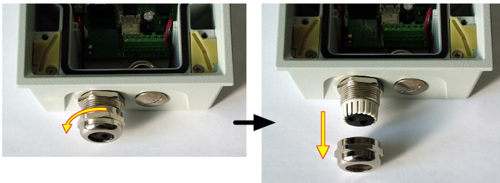
2. Remove the sealing including the cover from the bushing. Cut either of the components as shown in the figures.
