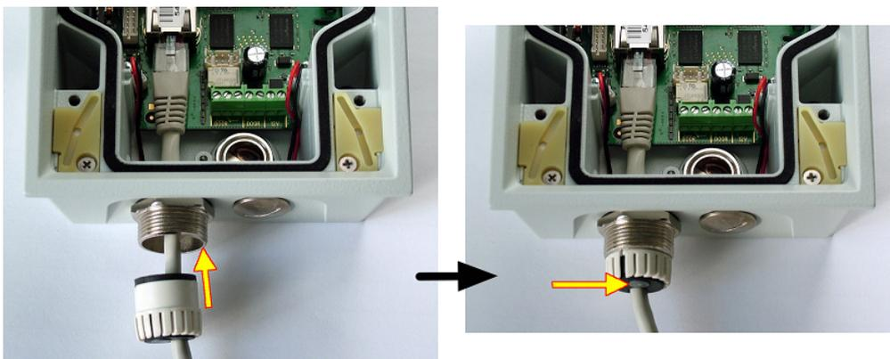
7. Replace and tighten the nut.
