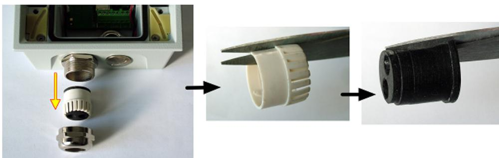
3. Put the bushing nut on the cable and insert the sealing.
