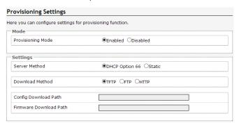
There are two different Provisioning methods that can be used: via DHCP Option 66 or via a Static Server. In addition, there are three different ways to download provisioning files from a "Provisioning Server": TFTP (Trivial File Transfer Protocol), FTP, or HTTP.
