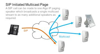
In the diagram above, the bottom 8180 is configured with a SIP Page Extension. When called from a phone, the SIP registered 8180 autoanswers and plays the page audio over its speaker. Simultaneously, the bottom 8180 broadcasts the audio over the network using multicast to as many additional 8180s as required (or 8188 ceiling speakers).
